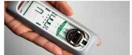
4. Replace the cover. Make sure to insert the upper part of the remote control first and then press the lower part closed.
