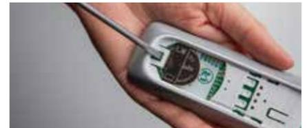
3. Insert a new battery (type CR 2430 3V) into the holder so that the side with the plus sign is visible. The connections must not be short-circuited. Push the battery into the compartment.
