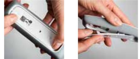
2. Push the empty battery out of the compartment with a plastic object or a screwdriver.
