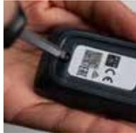
2. Push the empty battery out of the compartment with a plastic object or a screwdriver.
