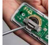
3. Insert a new battery (type CR 2032 3V) into the holder so that the side with the plus sign is visible. Take into account the polarity. The connections must not be short-circuited. Push the battery into the compartment.
