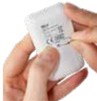
2. Remove the battery and replace it with one of the same type. Observe the polarity when inserting the new battery.
